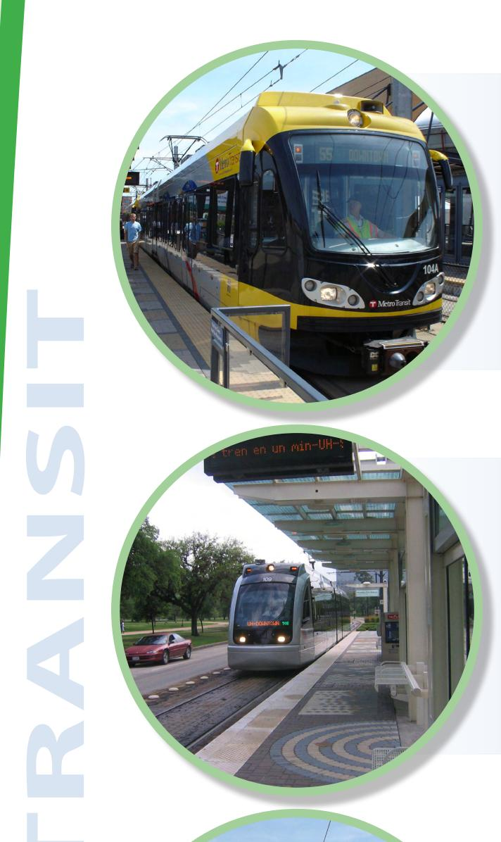
150 – 250 passengers Can operate in multiple car trains 100 – 150 passengers Typical single-car operation
